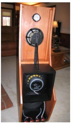
observed. The midrange and tweeter on-axis responses were outstandingly flat (+/- 3dB), well within my system's 1.5 dB accuracy window, up to the mid high-treble, where it showed the usual roll-off above 17 kHz. So the Orion gets completely right what many highend loudspeakers do not. The severe 45-degree off-axis response closely tracked to the on-axis response, only beginning to fall off at about 7 kHz. The vertical
